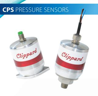
These piezoresistive silicone pressure sensors can either be used as feedback for the Cordis pressure controller or as standalone transducers. They are conditioned and offer a customized calibration around your specific application requirements, which allows for a full-scale accuracy of 0.25% over the calibrated range.
